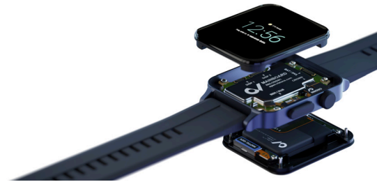
Ultracompact printed circuit boards are used in wearables such as smartwatches.
